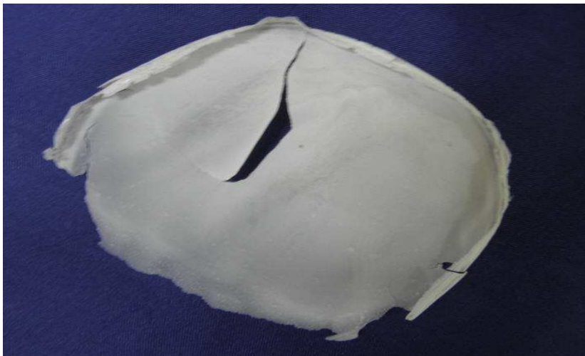
Fig. 9. Biopolymer of PHB obtained from Bacillus aryabhatai
