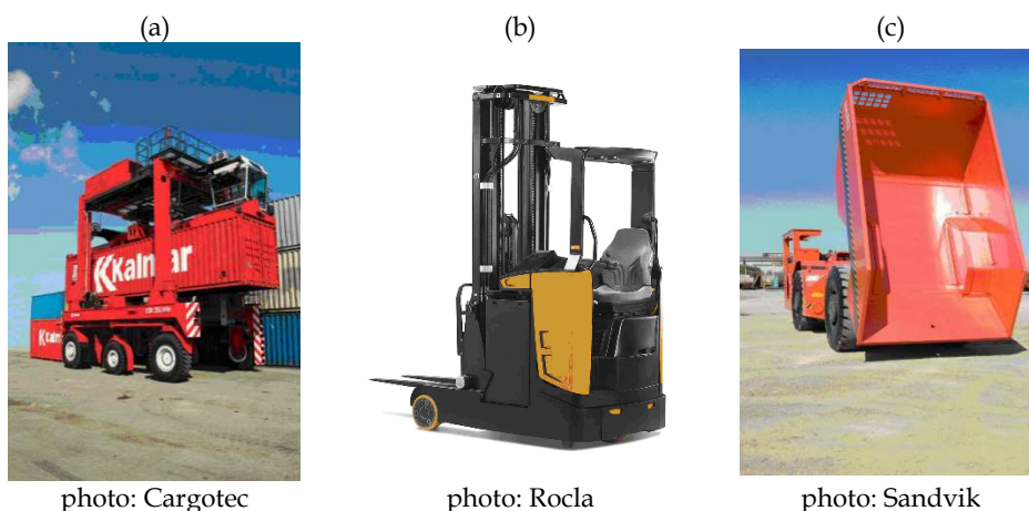
Fig. 1. Examples of mobile working machines: a) straddle carrier, b) forklift truck and c) mine underground truck. (Minav, 2011d)
