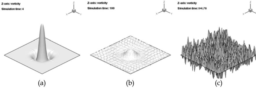
Fig. 3. Steady compressible Gaussian vortex in a periodic box domain: vorticity levels of the Roe-MUSCL solution on grid (240x240) cells with (a) MinMod limiter at time t=100, (b) MinMod limiter at time t=4, and (c) with the limiter deactivated at time t=5.
