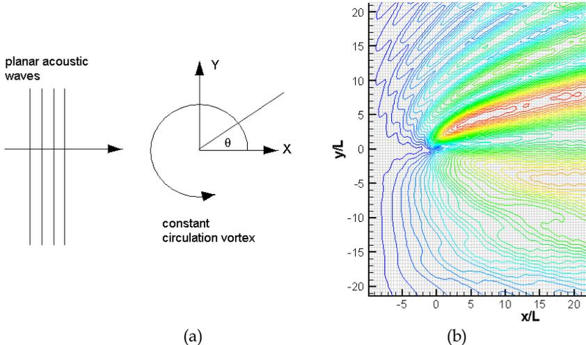
Fig. 4. Sound wave scattering by a non-zero circulation vortex of  $M=0.25$ : (a) problem configuration, (b) computed r.m.s of the scattered pressure field of the CABARET solution on coarse grid of 2.5 cells per vortex core radius.
