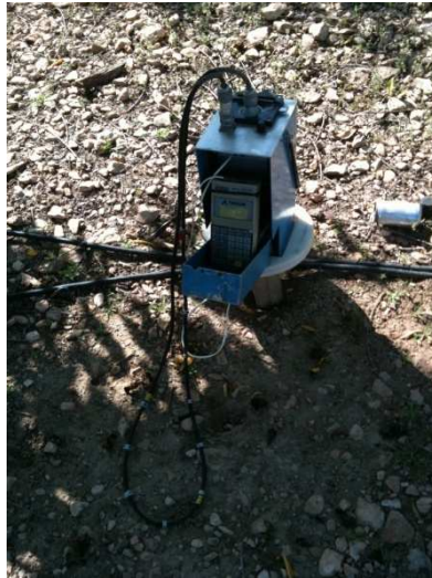
Fig. 3. Neutron probe for measuring soil water content.
