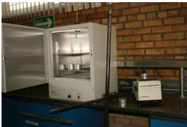
Fig. 2. Equipment used by the gravimetric technique for measuring soil water content.
