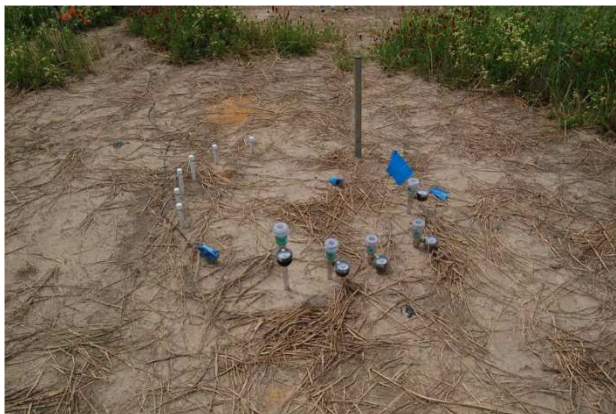
Fig. 5. Use of tensiometers to determine soil matric potential at different soil depths.
