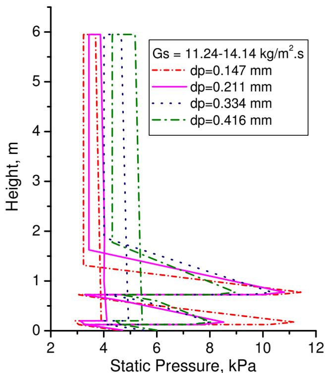
Fig. 8. Predicted pressure profiles in dual fluidized bed for sand # I, II, III and IV
