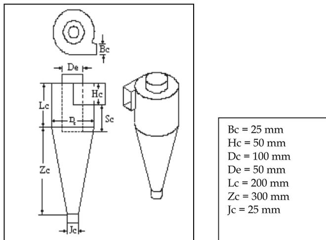
Fig. 2. Cyclone dimensions in dual FB system
