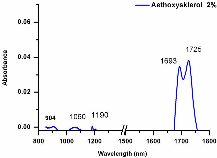
Fig. 8. NIR absorption spectrum of Aethoxysklerol 2%
