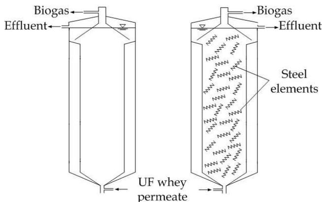
Fig. 1. Schematic of the laboratory-scale anaerobic treatment system
