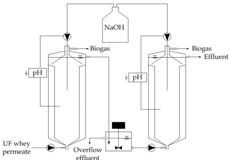
Fig. 12. Schematic of the two-stage fermentation system
