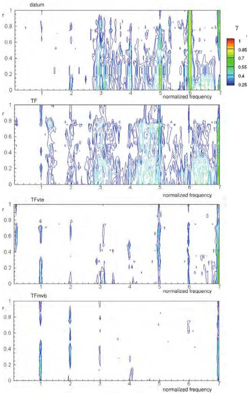
Fig. 8. Spanwise maps of coherence for the different blade geometries at 30°
