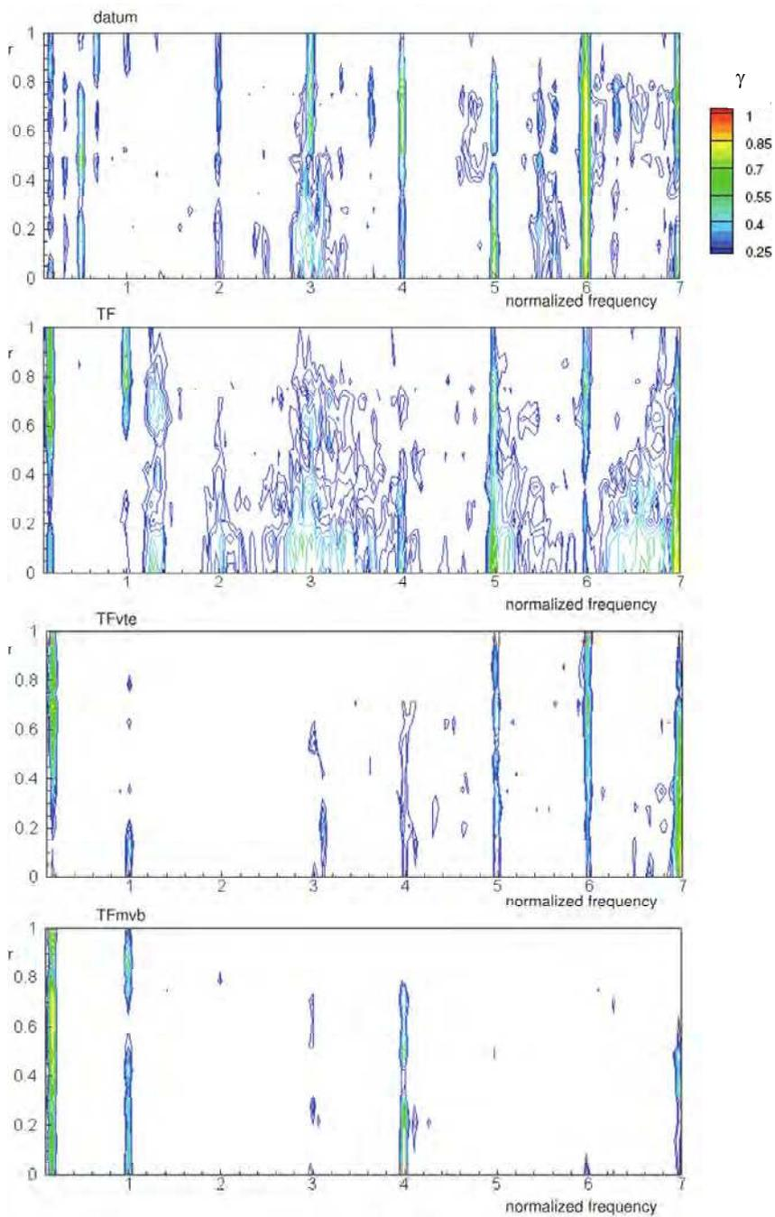
Fig. 9. Spanwise maps of coherence for the different blade geometries at 60°
