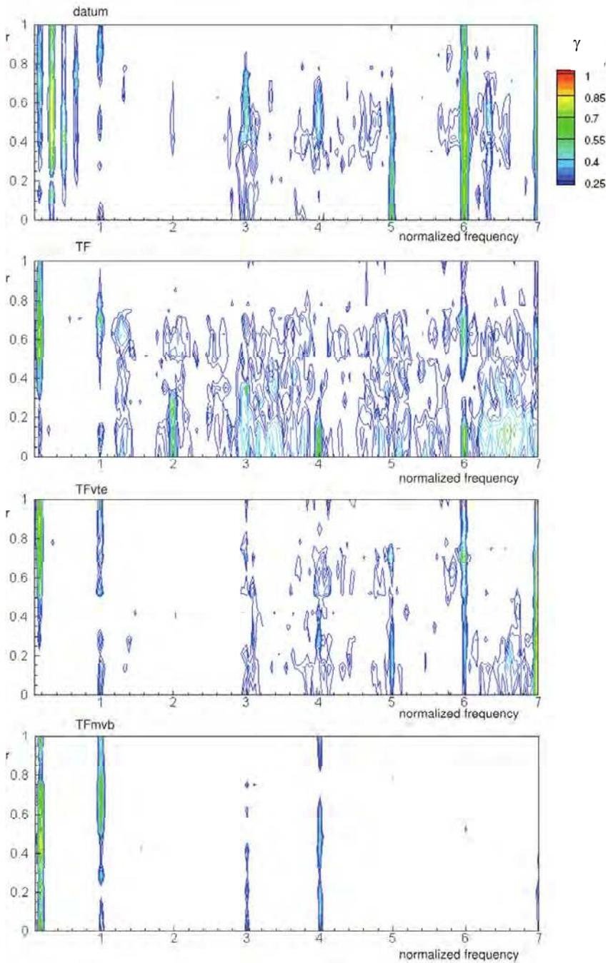
Fig. 10. Spanwise maps of coherence for the different blade geometries at 90°
