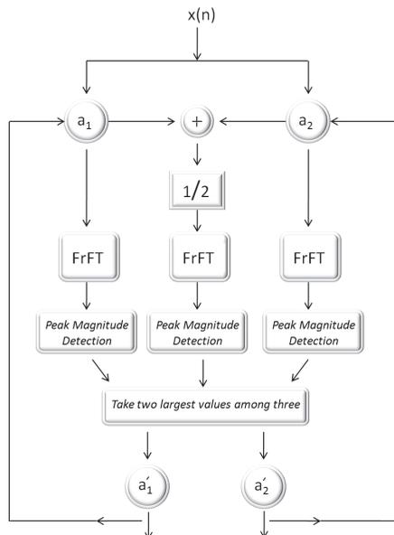
Fig. 4. A basic IF estimation scheme via RWT.
