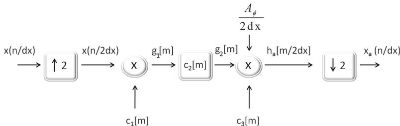
Fig. 2. The fast FrFT computation block diagram.
