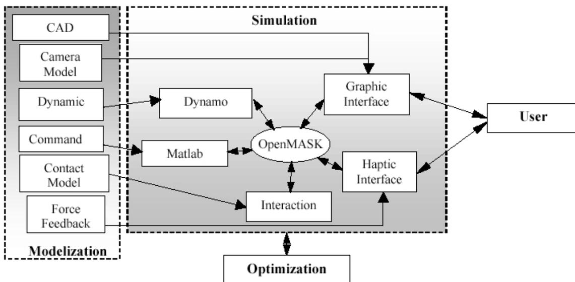
Figure 5. OpenMASK: Modular Animation and Simulation Kit
