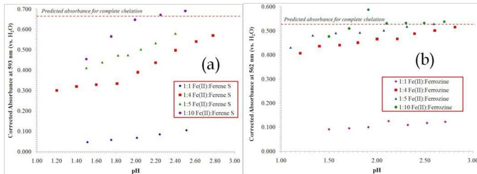
Fig. 6. Absorbance-pH formation curves for the spectrophotometric determination of the overall formation constant  $\beta_3$  for (a)  $\text{Fe}(\text{Ferene S})_3^{2+}$  and (b)  $\text{Fe}(\text{Ferrozine})_3^{2+}$  at varying  $\text{Fe}(\text{II})$ :ligand ratios.
