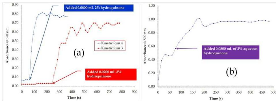
Fig. 8. Determination of (a) the amount of hydroquinone reducing agent to add for conversion of  $3.04 \times 10^{-5} \text{ mol Fe}^{3+} \text{ L}^{-1}$  solution to  $\text{Fe}^{2+}$ , and (b) the speciation of a synthetic sample containing  $2.95 \times 10^{-5} \text{ mol Fe}^{2+} \text{ L}^{-1}$  and  $1.52 \times 10^{-5} \text{ mol Fe}^{3+} \text{ L}^{-1}$ .
