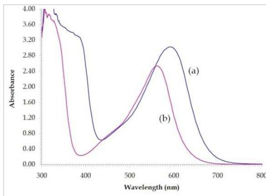
Fig. 3. The UV-visible spectra of (a)  $\text{Fe}(\text{Ferene S})_3^{2+}$ ,  $1.00 \times 10^{-4} \text{ mol L}^{-1}$ , and (b)  $\text{Fe}(\text{Ferrozine})_3^{2+}$ ,  $1.00 \times 10^{-4} \text{ mol L}^{-1}$ .
