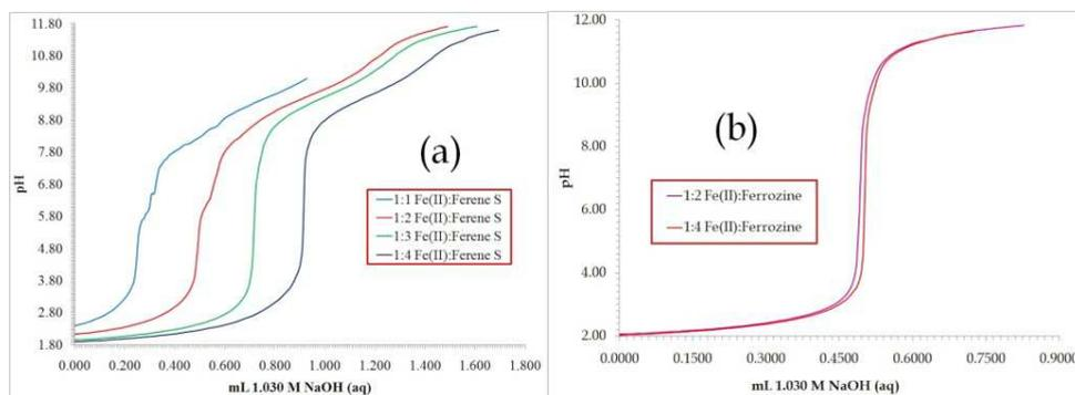
Fig. 7. pH titration curves for (a)  $\text{Fe}(\text{Ferene S})_3^{2+}$  at  $\text{Fe}(\text{II})$ : $\text{Ferene S}$  ratios of 1:1 through 1:4, and (b)  $\text{Fe}(\text{Ferrozine})_3^{2+}$  at  $\text{Fe}(\text{II})$ : $\text{Ferrozine}$  ratios of 1:2 and 1:4.
