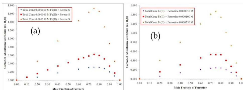
Fig. 5. Continuous variation plots for (a)  $\text{Fe}(\text{Ferene S})_3^{2+}$  and (b)  $\text{Fe}(\text{Ferrozine})_3^{2+}$ , at three different total concentrations of Fe(II) + ligand (in mol L<sup>-1</sup>).
