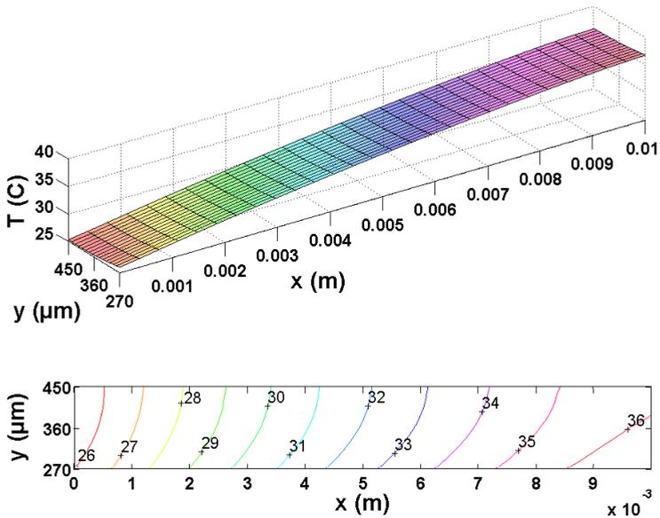
Fig. 23. Numerical predictions of local temperature distribution in the unit cell side walls.
