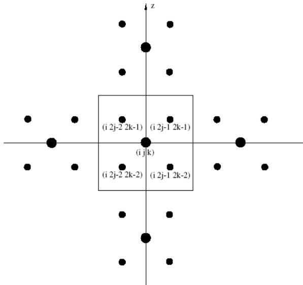
Fig. 4. Schematic of a cell-centered two-level multigrid configuration.
