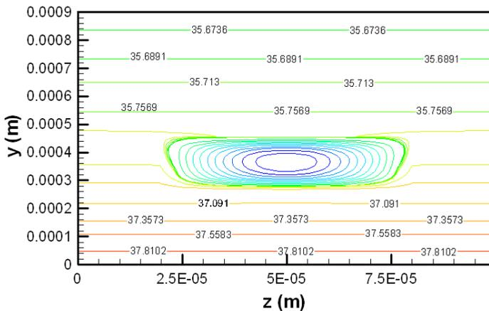
Fig. 16. Contour of temperature in the heat sink at the cross-section of the outlet of the channel ( $\Delta p = 50 \text{ kPa}$ ,  $Re = 162.68$ ,  $T_{reference} = 32^\circ\text{C}$ ,  $u_m = 1.44 \text{ m/s}$ ).
