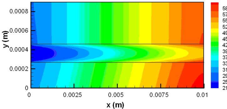
Fig. 19. Local temperature distribution in  $x$ - $y$  plane at  $z=L_z/2$  ( $\Delta p=15$  kPa,  $Re=85.60$ ,  $T_{reference}=48^{\circ}C$ ,  $u_m=0.57$  m/s).
