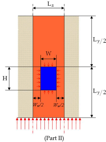
Fig. 1. Schematic of a rectangle microchannel heat sink and the unit cell.
