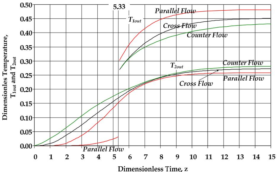
Fig. 7. Outlet Temperature of Both Fluids for Parallel, Counter and Cross Flow Heat Exchangers.
