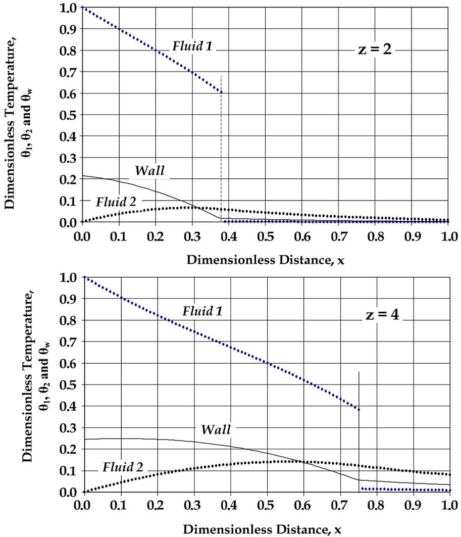
Fig. 4. Temperature Distribution of Both Fluids and the Wall of Parallel Flow Heat Exchanger for  $z = 2$  and 4.
