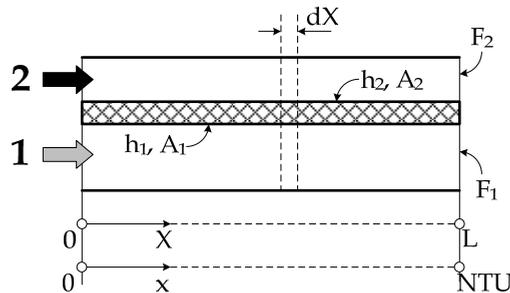
Fig. 1. Schematic Description of Parallel Flow Heat Exchanger.
