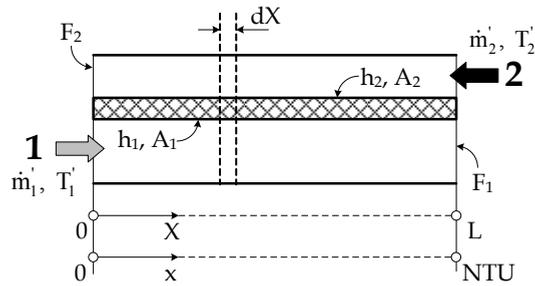
Fig. 2. Schematic Description of Counter Flow Heat Exchanger
