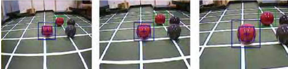
Figure 7. 3-D tracking of red balls. A camera is mounted on a wheeled robot which is moving in the ground plane (basketball robot players). Given the radius, red balls should be tracked and picked up
