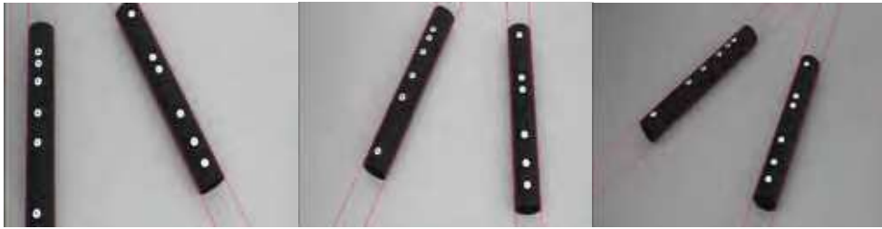
Figure 9. The 3-D tracking of the cylinder's axis through the detection of the conjugate apparent lines in a uniform background
