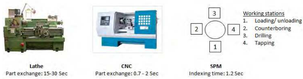
Fig. 17. Part exchange time on traditional lathe, CNC, and SPM.
