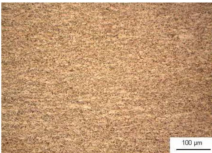
Fig. 14. Microstructure of HSn (magnified 200 times).
