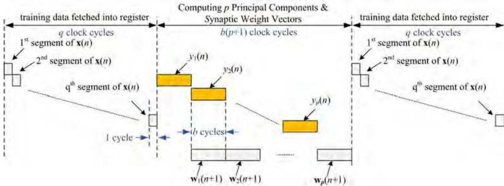
Fig. 13. The timing diagram of the proposed architecture.
