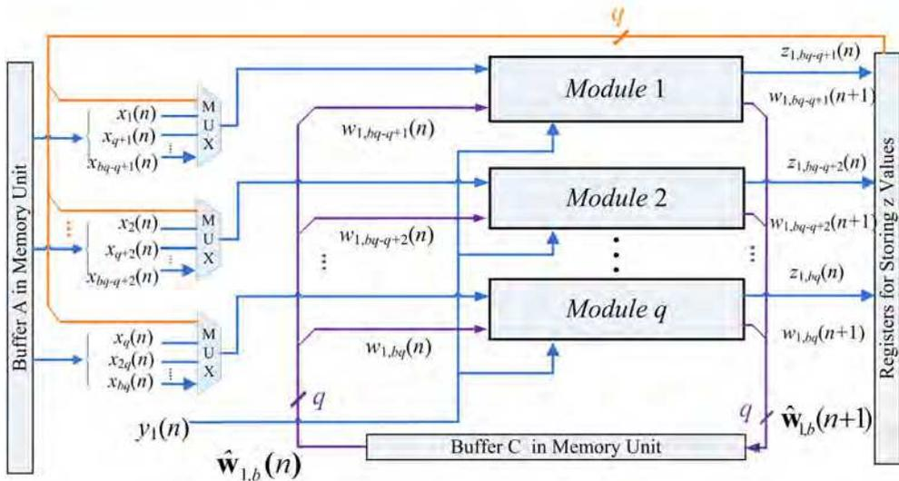
Fig. 7. The operation of SWU unit for computing the  $b$ -th segment of  $w_1(n+1)$ .
