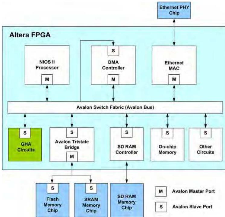
Fig. 14. The SOPC system for implementing GHA.
