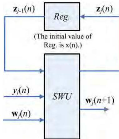
Fig. 3. The hardware implementation of eqs.(5) and (6).
