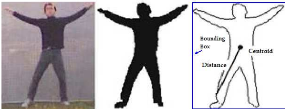
Fig. 2. Blob representation by means of a bounding box.
