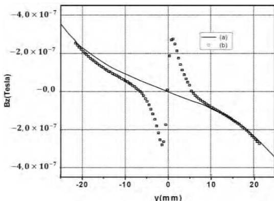
Fig. 11. Measured values of  $B_z$ , with a Hall probe at  $d = 1mm$  above the plate, between  $A$  and  $A'$ : (a) in the case of a defect free rectangular aluminium plate, (b) in the case of a rectangular plate with a slot of zero width
