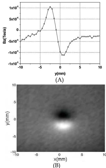
Fig. 17. (A) Measured values of  $B_z$  along the  $Oy$  axis for  $x = 0$  mm, (B) matrix representation of the values of  $B_z$  across a square domain ( $-10mm \leq x, y \leq +10mm$ ). Measurement with a Hall probe at  $d=1$ mm above the square aluminium plate ( $D = 4$ mm,  $d = 0.11$ mm)
