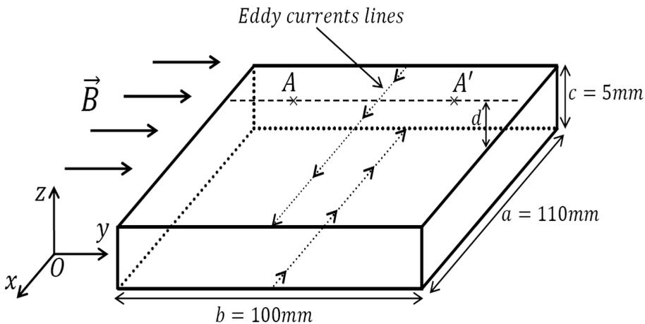
Fig. 1. Defect free rectangular aluminium plate under consideration
