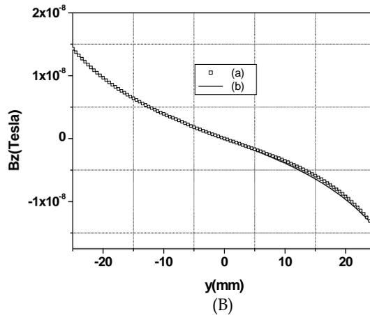
Fig. 9. Computed (a) and measured (b) values of  $B_z$  between  $A$  and  $A'$  in the case of a defect free rectangular aluminium plate: (A) measurement with a Hall probe at  $d = 1\text{mm}$  above the plate, (B) measurement with a SQUID at  $d = 12.8\text{mm}$  above the plate
