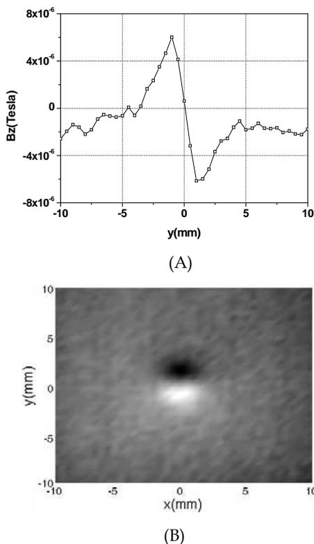
Fig. 18. (A) Measured values of  $B_z$  along the  $Oy$  axis for  $x = 0\text{ mm}$ , (B) matrix representation of the values of  $B_z$  across a square domain ( $-10\text{ mm} \leq x, y \leq +10\text{ mm}$ ). Measurement with a Hall probe at  $d=1\text{ mm}$  above the square aluminium plate ( $D = 3\text{ mm}$ ,  $d = 0.09\text{ mm}$ )
