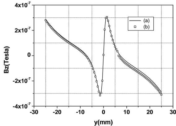
Fig. 13. (a) Theoretical curve with optimized values of  $w' = 50\mu m$  and  $\rho' = 1.5 \times \rho$ , (b) experimental curve established with a Hall sensor at  $d=1mm$  above the aluminium plate in the case of a zero width crack
