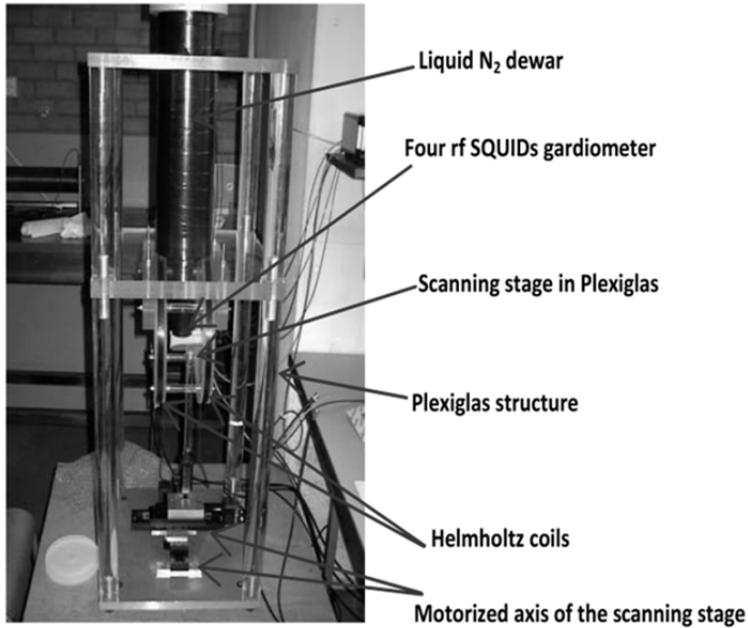
Fig. 5. High T<sub>c</sub> SQUID NDE instrumentation set-up
