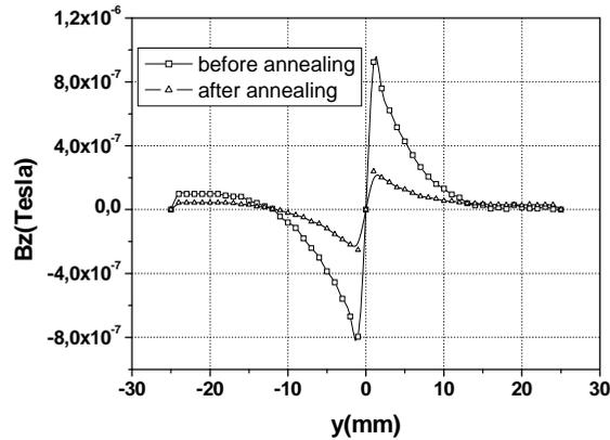
Fig. 15. Experimental curve established with a Hall sensor at  $d=1\text{mm}$  above the aluminium plate in the case of a zero width crack before and after annealing
