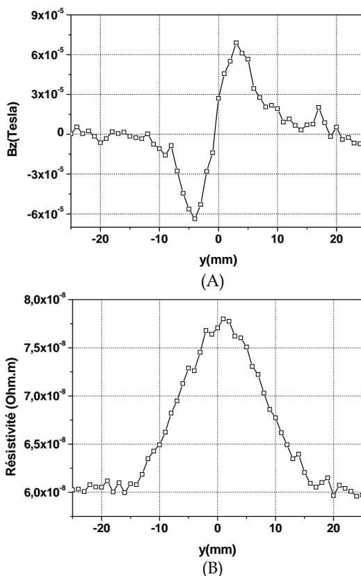
Fig. 23. (A) Values of  $B_z$  induced by the eddy currents within a flattened fatigued long strip (measurement with a Hall sensor at  $d = 1\text{mm}$  above the strip), (B) Corresponding values of the estimated local resistivity along the damaged zone using the inverse solution
