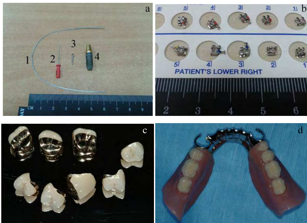
Fig. 1. a) Representative examples of industrially-made dental devices: 1) orthodontic archwire made of Ni-Ti alloy, 2) endodontic file made from Ni-Ti alloy, 3) Mini-orthodontic implant made of cp-Ti and 4) dental implant made of Ti. b) Industrially-made orthodontic brackets fabricated from stainless steel alloy. c) Custom-made ceramo-metal crowns. d) Custom made removable partial denture made of Cr-Co alloy and acrylic resin.
