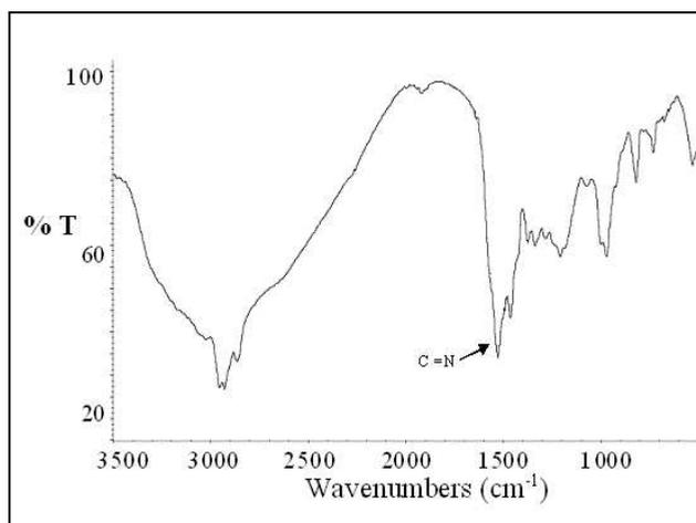
Fig. 4. FT-IR spectrum of polyoxadiazole, PThOxad 1c.
