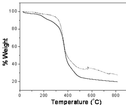
Fig. 9. TGA graphs for PThOxad 3c (—) and PThOxad 3c/TiO<sub>2</sub> nanocomposite (---).
