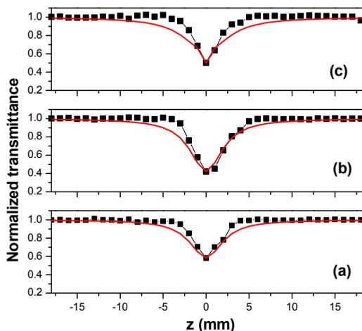
Fig. 13. Open aperture curves for PThOxad 1a (a), PThOxad 1b (b) and PThOxad 1c (c). Solid line is a fit of data to equation (1) assuming only 2PA, with  $\beta = 73.8$  cm/GW for PThOxad 1a,  $\beta = 53$  cm/GW for PThOxad 1b and  $\beta = 63.6$  cm/GW for PThOxad 1c.
