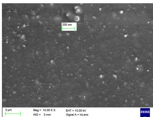
Fig. 10. SEM images of PThOxad 3c/TiO<sub>2</sub> nanocomposite (Inset: magnified image, Mag. = 100 K X).
