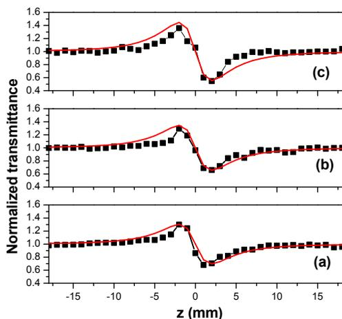
Fig. 16. Pure nonlinear refraction curve obtained for PThOxad 1a (a), PThOxad 1b (b) and PThOxad 1c (c). Solid lines are fit of data to equation (3) with  $\Delta\Phi_0 = 1.5$  for PThOxad 1a,  $\Delta\Phi_0 = 1.7$  for PThOxad 1b and  $\Delta\Phi_0 = 2.2$  for PThOxad 1c.
