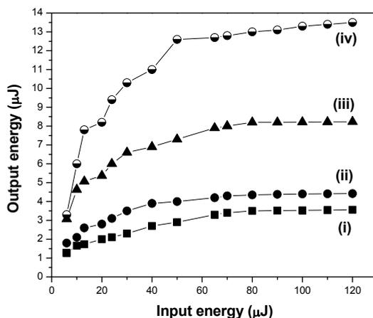
Fig. 19. Optical limiting behaviors of PThOxad 1a-c at different concentrations: (i)  $1 \times 10^{-5}$  Mol/L; (ii)  $0.5 \times 10^{-5}$  Mol/L; (iii)  $0.25 \times 10^{-5}$  Mol/L; (iv)  $0.125 \times 10^{-5}$  Mol/L.
