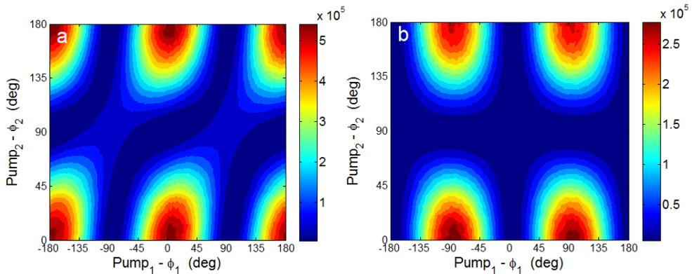
Fig. 5. Noncollinear second harmonic signal experimentally measured as a function of the polarization state of the first pump beam ( $\phi_1$ ) and the second pump beam ( $\phi_2$ ). Sample rotation angle was fixed to  $\alpha=9^\circ$ . The polarization state of the analyzer is set to (a)  $\hat{p}$  i.e.  $\phi=0^\circ$  and (b)  $\hat{s}$ , i.e.  $\phi=90^\circ$ .
