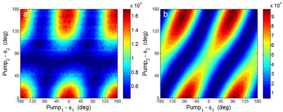
Fig. 4. Noncollinear second harmonic signal experimentally measured as a function of the polarization state of the first pump beam ( $\phi_1$ ) and the second pump beam ( $\phi_2$ ). Sample rotation angle was fixed to  $\alpha=1^\circ$ . The polarization state of the analyzer is set to (a)  $\hat{p}$  i.e.  $\phi=0^\circ$  and (b)  $\hat{s}$ , i.e.  $\phi=90^\circ$ .
