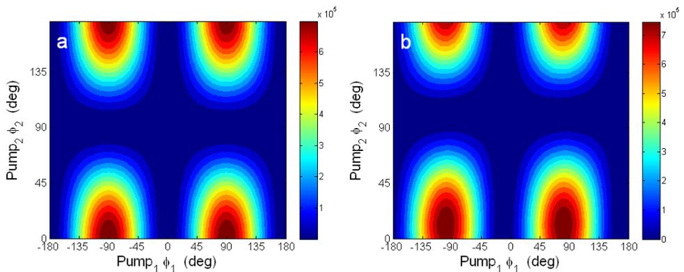
Fig. 7. Theoretically calculated curves of  $\hat{s}$ -polarized second harmonic signal as a function of the polarization angle of the first pump beam ( $\phi_1$ ) and the second pump beam ( $\phi_2$ ), calculated for the optical axis (a) normal to the sample surface and (b) tilted about the x-axis of 2 degrees. Sample rotation angle is  $\alpha=9^\circ$ .
