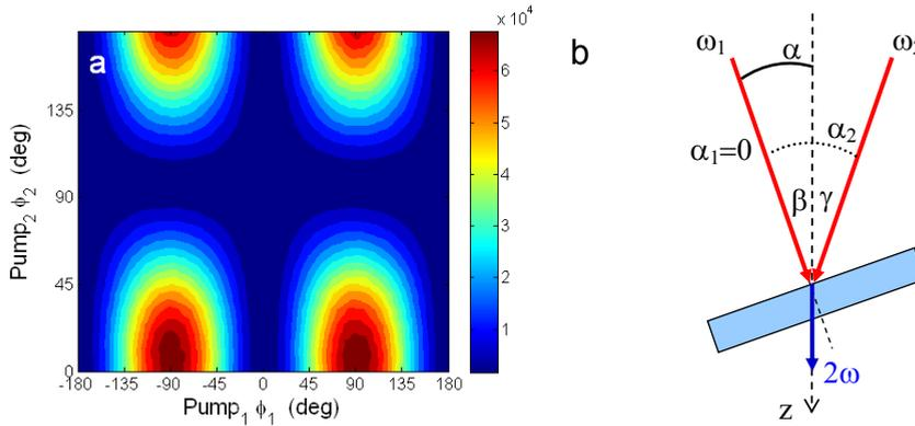
Fig. 6. (a) Noncollinear SH signal measured as a function of the polarization state of the first pump beam ( $\phi_1$ ) and the second pump beam ( $\phi_2$ ).The polarization state of the analyzer is set to  $\hat{s}$ , i.e.  $\phi=90^\circ$ . (b) Sketch of the experimental configuration: sample rotation angle was fixed to  $\alpha=9^\circ$ .
