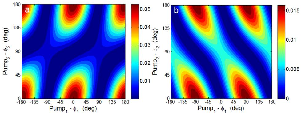
Fig. 3. Noncollinear second harmonic signal theoretically calculated as a function of the polarization state of the first pump beam ( $\phi_1$ ) and the second pump beam ( $\phi_2$ ). Sample rotation angle was fixed to  $\alpha=35^\circ$ . The polarization state of the analyzer is set to (a)  $\hat{p}$  i.e.  $\phi=0^\circ$  and (b)  $\hat{s}$ , i.e.  $\phi=90^\circ$ .
