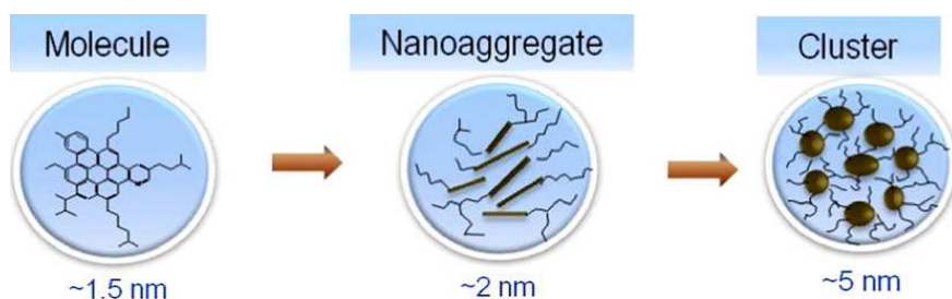
Fig. 11. The modified Yen model. Courtesy of O. Mullins, Schlumberger
