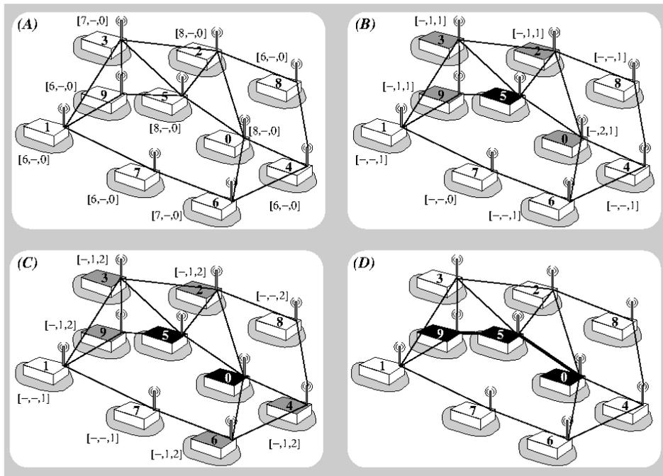
Fig. 3. Example (2,2)-CDS applying the centralized solution
