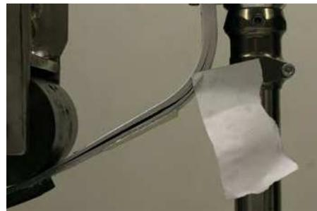
(b) Left side of the split-toe foot under static loading.
