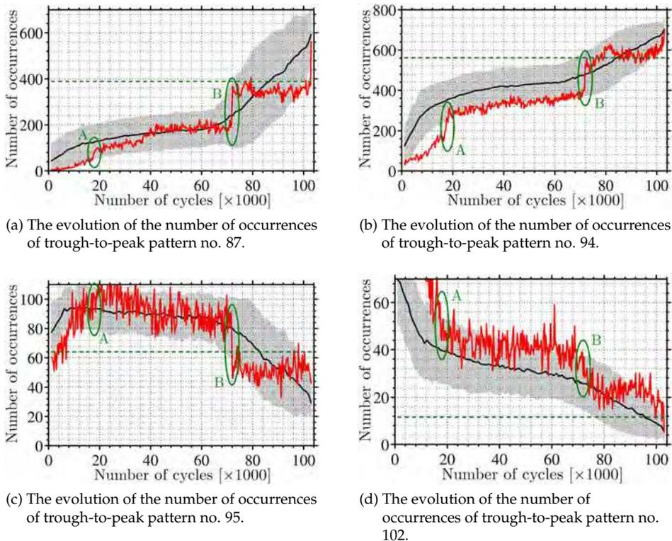
Fig. 11. The evolution of the number of occurrences for four trough-to-peak (ISI) patterns computed from the AE segments. The grey area for each pattern represents all values which lie within one standard deviation from the mean (black curve). The mean is computed by averaging the evolution curves from all other feet.
