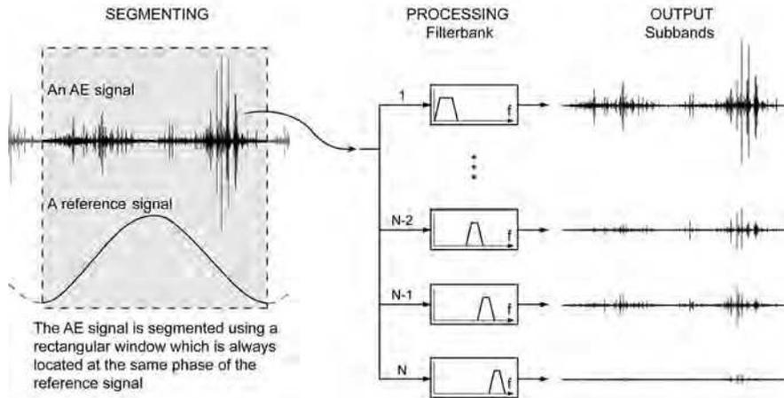
Fig. 2. Illustration of how the AE signal is segmented using a reference signal and then split into  $N$  subbands. All segments start at the same phase of the reference signal and are exactly one cycle.
