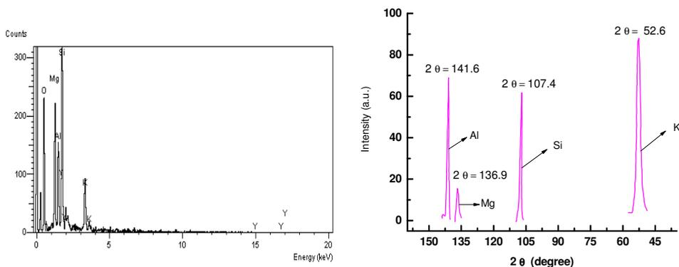
Fig. 19. (a-b): Chemical composition analysis of MAS-G8 (a) EPMA spectra (b) XRF patterns.
