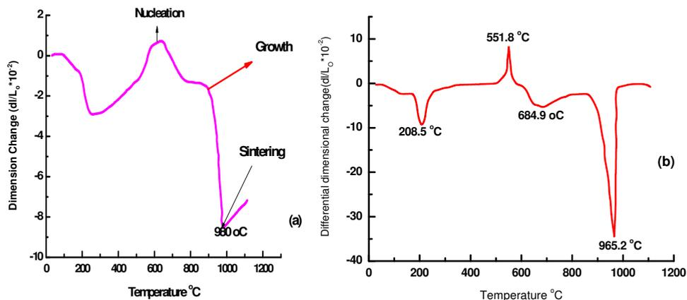
Fig. 7. (a-b): Thermodilatometric (a) and differential dilatometric (b) curves of green compact of magnesium aluminum silicate glass ceramic specimen MAS-G4.
