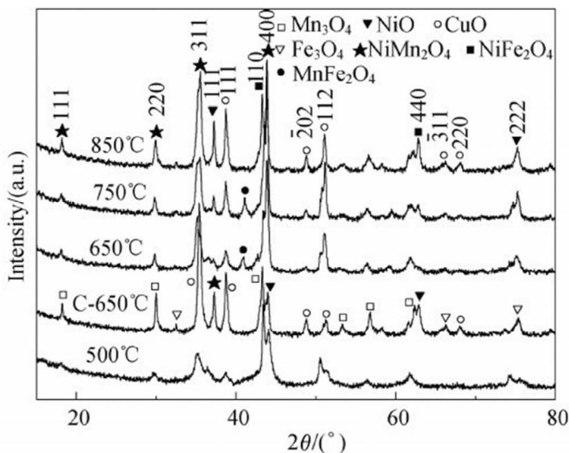
Fig. 1. XRD patterns of  $\text{Mn}_{0.43}\text{Ni}_{0.9}\text{CuFe}_{0.67}\text{O}_4$  powder calcined at different temperature 500–850°C: microwave sintering with dwelling time of 30min; C-650°C: conventionally calcined at 650°C[12].
