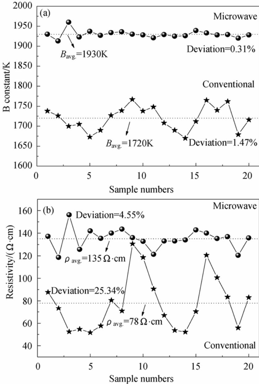
Fig. 4. Distribution of (a) B constant, (b) ρ for twenty components[12].
