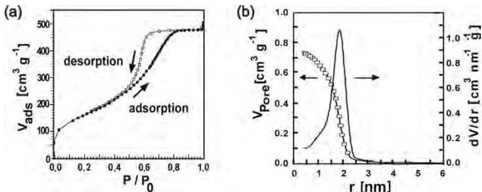
Fig. 13. BET nitrogen adsorption-desorption isotherm of the platinum doped silica catalyst microspheres produced through our microfluidic reaction scheme.  $V_{ads}$  = adsorbed volume,  $p/p_0$  = reduced pressure.
