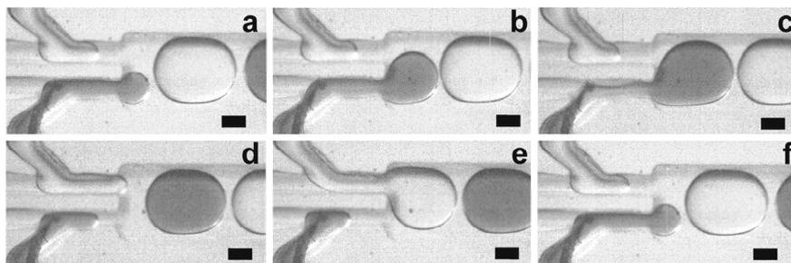
Fig. 4. (a) Schematic of the double step-emulsification device. The typical device dimensions were  $a = b = 35 \mu\text{m}$ ,  $H = 120 \mu\text{m}$  and  $W = 160 \mu\text{m}$ . (b) Time series of optical images showing the droplet formation using a double step-emulsification device. For clarity, the aqueous phase injected from bottom is dyed with Nile blue. Scale bar:  $50 \mu\text{m}$ .
