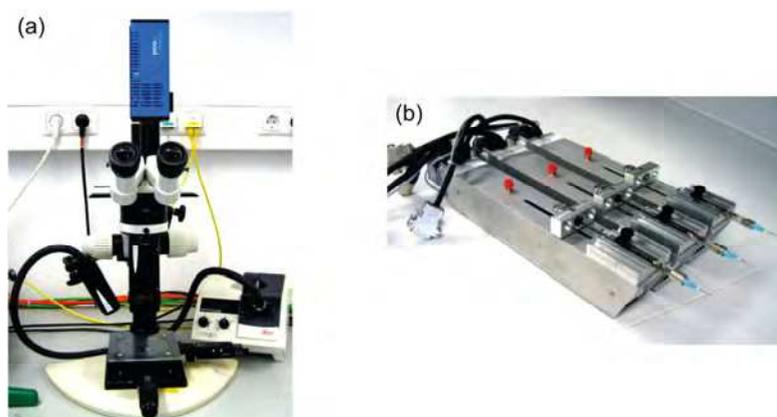
Fig. 3. a) Leica macroscope Z16 APO with a Leica L5 FL light source and camera. b) Custom made syringe pumps with glass syringes (Hamilton).
