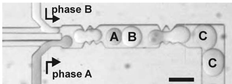
Fig. 6. Optical micrograph showing the production of droplets *A* and *B* having different volumes, the formation of separated droplet pairs lead by the bigger droplet and the subsequent coalescence into droplets *C* at a geometrical constriction. The aqueous phase injected from the bottom channel is colored with Nile blue for clarity. Scale bar: 200  $\mu\text{m}$ .
