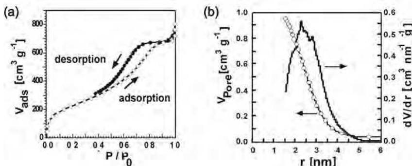
Fig. 11. (a) BET nitrogen adsorption-desorption isotherm of the produced silica spheres.  $V_{\text{ads}}$  = adsorbed volume,  $p/p_0$  = reduced pressure (b) Pore size distribution.  $V_{\text{pore}}$  = pore volume,  $r$  = pore radius.
