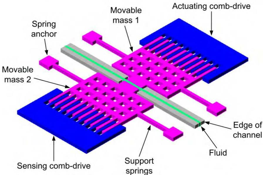
Fig. 1. A schematic of the coupled-mass microrheometer
