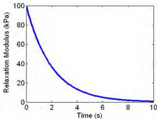
Fig. 7. Typical relaxation data for a simple Maxwell fluid
