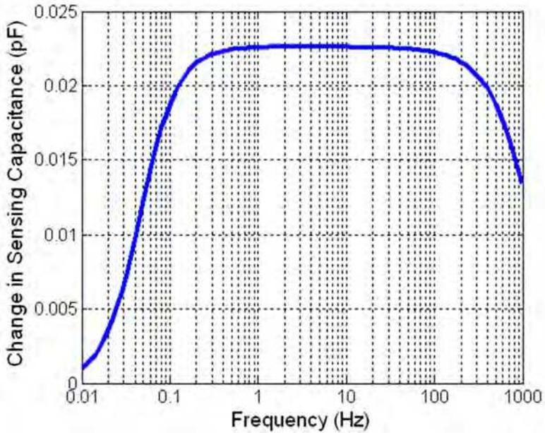
Fig. 10. Resultant change in amplitude of capacitance of sensing comb-drive
