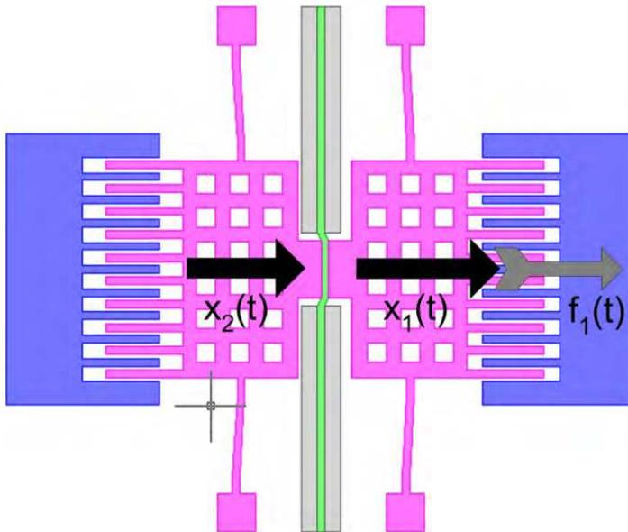
Fig. 2. A schematic showing the dynamics of the microrheometer. Here  $x(t)$  denotes the displacement of each of the masses respectively and  $f_1(t)$  denotes the force applied by the actuating comb drive
