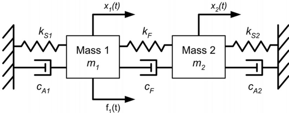
Fig. 3. A schematic of the equivalent lumped-mass system.  $k_S$  and  $c_A$  denote the stiffness of the support springs and the air damping associated with each of the masses,  $m$ .  $k_F$  and  $c_F$  denote the effective stiffness and damping parameters which are a function of the fluids viscoelastic properties
