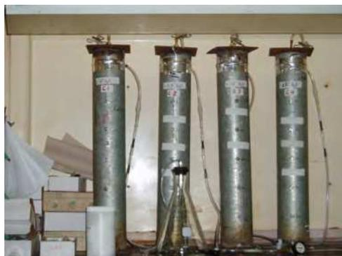
Fig. 1a. Soil columns with charcoal filters.
