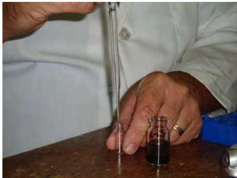
Fig. 3b. Transfer of solvent to small GC vial.
