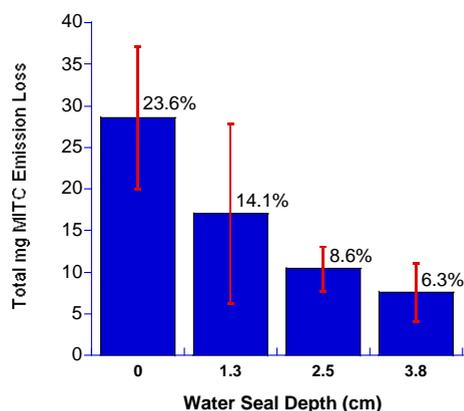
Fig. 6a. Mean MITC emitted from soil columns.
