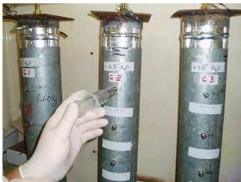
Fig. 1b. MS injection at 15 cm soil depth.
