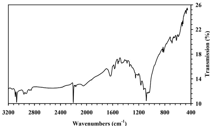
Fig. 7. Infrared spectrum at 298 K for TTF·TCNQ nanoparticles dispersed in KBr matrix (mean diameter: 35 nm; stabilizing agent: BMIMBF<sub>4</sub>)
