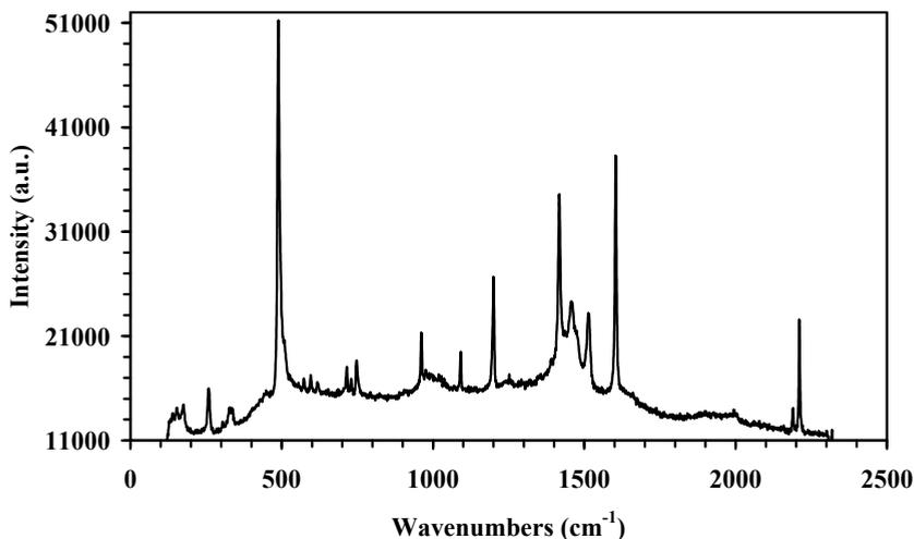
Fig. 8. Raman spectrum at 77 K for TTF·TCNQ as a nanoparticle film (mean diameter of individual particles: 35 nm; stabilizing agent: BMIMBF<sub>4</sub>)
