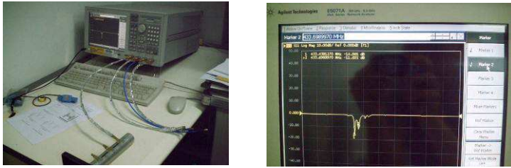
Fig. 31. Torque measurement using the network analyzer (Agilent E5071A).
