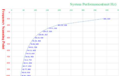
Fig. 45. Number of frequency scanning points v.s. the system bandwidth.
