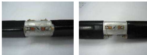
Fig. 35. The rotational shaft equipped with two SAWRs.
