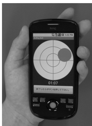
Fig. 2. An Android application allows users to control the position of a small blue circle (1.5 cm in diameter) on a large white circle (4 cm in diameter). Scores are automatically calculated on the basis of coordinate tracking data for the blue circle.
