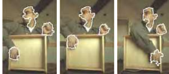
Figure 7. A few frames of the captured video overlaid with the object region borders (in white), as detected by the stereo tracking algorithm
