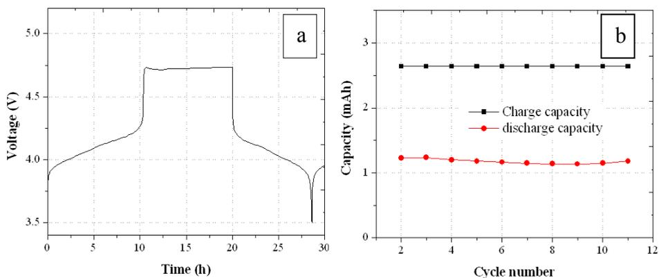
Fig. 8. a) Representative cell voltage *vs.* time for  $\text{LiMn}_2\text{O}_4/\text{Li}$  cell containing 5 wt% TEDBPDP; b) cell charge-discharge capacities *vs.* cycle number in overcharge test. Cells were charged at C/10 rate for 20 h and then discharged at C/10 rate.
