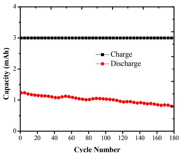
Fig. 12. Capacity retention profiles of MCMB/LiFePO<sub>4</sub> containing 0.4 M ANL-2 in Gen 2 electrolyte. Charging rate is C/2, and overcharge ratio is 100%.
