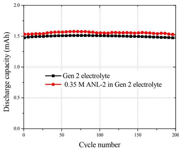
Fig. 13. Capacity retention profiles of MCMB/LiFePO<sub>4</sub> cells containing Gen 2 electrolyte with and without 0.35 M ANL-2 additive. Charging rate is C/3, and cut-off voltage is 2.3 ~3.6 V.
