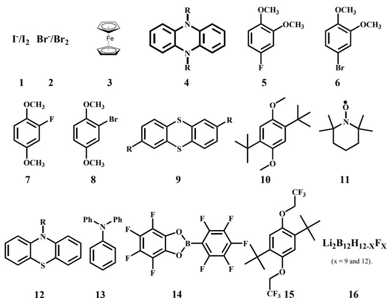
Fig. 2. Representative examples of redox shuttle additives
