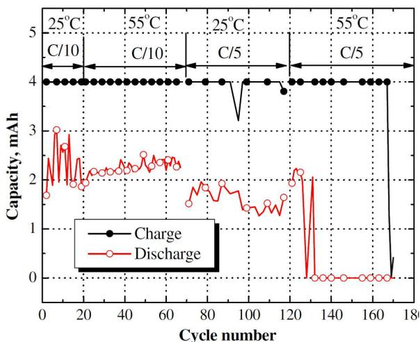
Fig. 5. Charge and discharge capacity of graphite/ $\text{LiNi}_{0.8}\text{Co}_{0.15}\text{Al}_{0.05}\text{O}_2$  cell during the whole course of overcharge test. The electrolyte used contained 5 wt% PFPTFBB. (Reprinted from *Electrochem. Commun.*, 9: 703–707, Copyright (2007), with permission from Elsevier).
