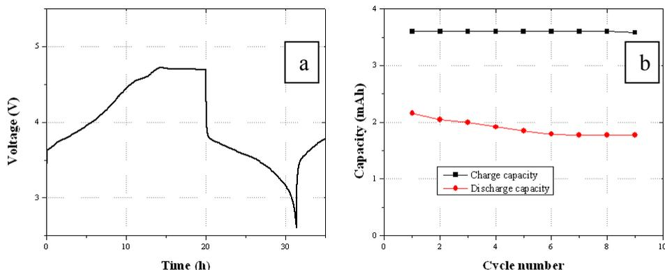
Fig. 9. a) Representative cell voltage *vs.* time for Li/Li<sub>1.2</sub>Ni<sub>0.15</sub>Co<sub>0.1</sub>Mn<sub>0.55</sub>O<sub>2</sub> cell containing 5 wt% TEDBPDP; b) cell charge-discharge capacities *vs.* cycle number in overcharge test. Cells were charged at C/10 rate for 20 h and then discharged at C/10 rate.
