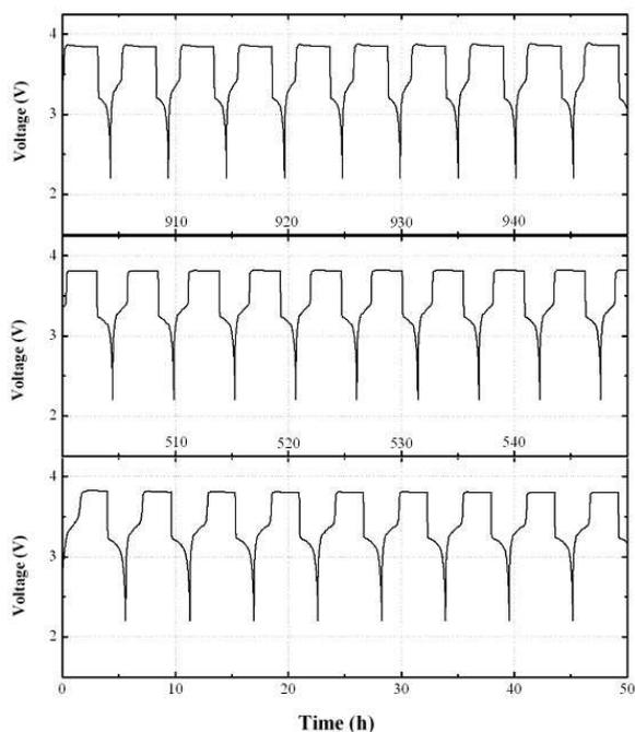
Fig. 11. Voltage profiles of MCMB/LiFePO<sub>4</sub> cells containing 0.4 M ANL-2 in Gen 2 electrolyte during 960-h overcharge test. Charging rate is C/2, and overcharge ratio is 100%.
