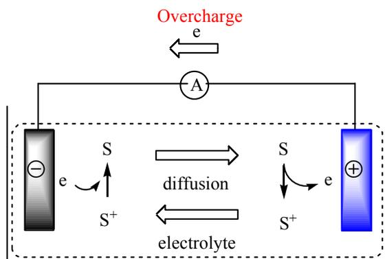
Fig. 1. Mechanism of redox shuttle overcharge protection
