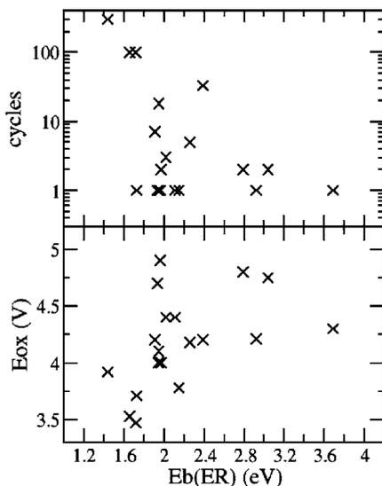
Fig. 3. Number of shuttle protected overcharge cycles sustained and the oxidation potentials of 19 shuttle molecules as a function of their binding energies with C<sub>2</sub>H<sub>5</sub>. (Reprinted from Journal of the Electrochemical Society, 2006, 153, A1922, Copyright (2006), with permission from the Electrochemical Society.)
