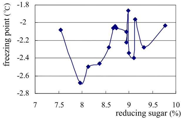
Fig. 3. freezing point of Kiwi vs. reducing sugar
