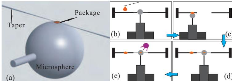
Fig. 8. (a) The schematic diagram of the spot-packaged microsphere-taper coupling system. (b)-(e) Illustration of the spot-package process. Red color represents the package glue.
