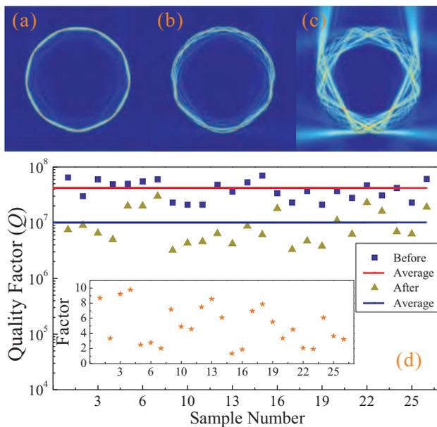
Fig. 10. (a), (b) and (c) The electric intensity distribution of three typical modes in the spot-packaged microsphere. (d) Tested  $Q$  of different microspheres before and after the spot-package. Inset: The decreased factor of the  $Q$  corresponds to different samples.
