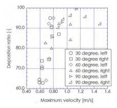
Fig. 24. Correlation analysis between deposition ratio and maximum velocity
