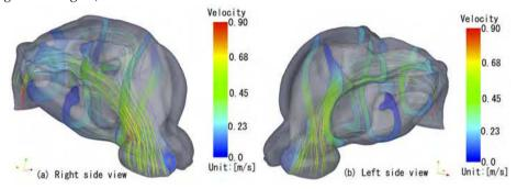
Fig. 21. Trajectories of nebulizer droplets of the case-III; inflow velocity of 0.5m/s and inlet angle of 60 degree)
