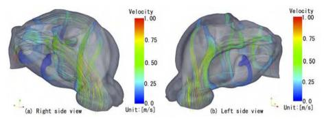
Fig. 20. Trajectories of nebulizer droplets of the case-III; inflow velocity of 0.5m/s and inlet angle of 90 degree)
