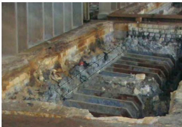
Fig. 19. Damaged back wall of an industrial magnesium electrolyzer due to the frequently washing of the small electrolyte circulation
