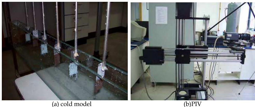
Fig. 2. Cold model experiment and PIV instrument
