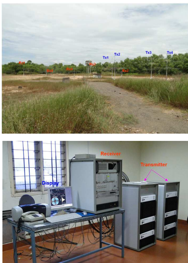
Fig. 2. Panoramic view of transmitter/receiver antenna system (top panel) and in-house transmitter/receiver system of SKiYMET meteor wind radar at Thumba.
