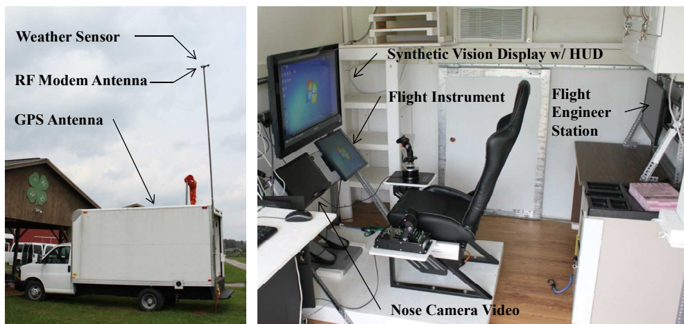
Fig. 4. The exterior (left) and interior (right) of the ground control station vehicle.
