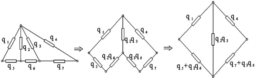
Fig. 4. Successive transformation of the electromagnetic system – example 3.
