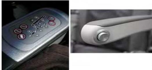
Fig. 3. Electronic Vs Mechanical seat adjustment
