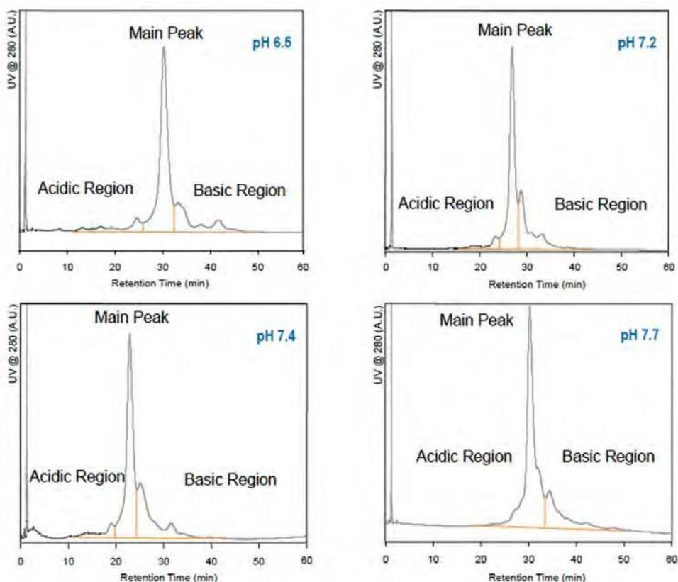
Fig. 7. Effect of mobile phase pH on mAb separation by WCX. The elution buffer (0.5 M NaCl) was increased linearly at  $1 \text{ mM min}^{-1}$  at a flow rate of  $1 \text{ mL min}^{-1}$  on a ProPac WCX-10 column ( $4 \times 250 \text{ mm}$ ), which was held at  $30^\circ\text{C}$ . Different initial salt concentrations were optimized for each pH value. Integration is shown, and main peak, acidic and basic regions are denoted.
