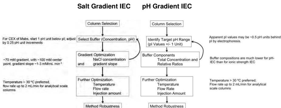
Fig. 5. Sequential salt-gradient IEC and pH-gradient IEC method development and optimization work flow.
