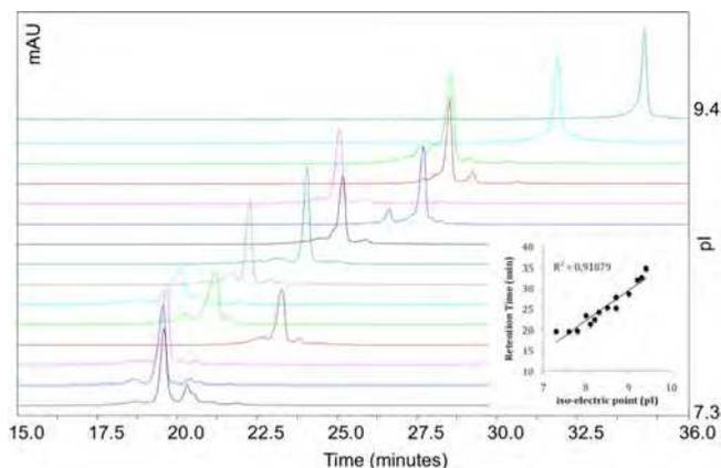
Fig. 9. Separation of 16 mAbs using a ProPac WCX-10 column by pH gradient IEC. Each mAb was analyzed using the same pH-IEC method, and each mAb was injected sequentially. mAb pI values ranged from pI 7.3 to pI 9.4.
