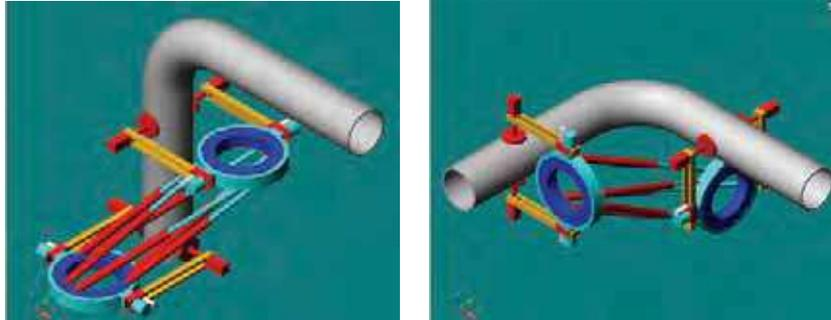
Fig. 7. Parallel robot climbing outside tubular structures.
