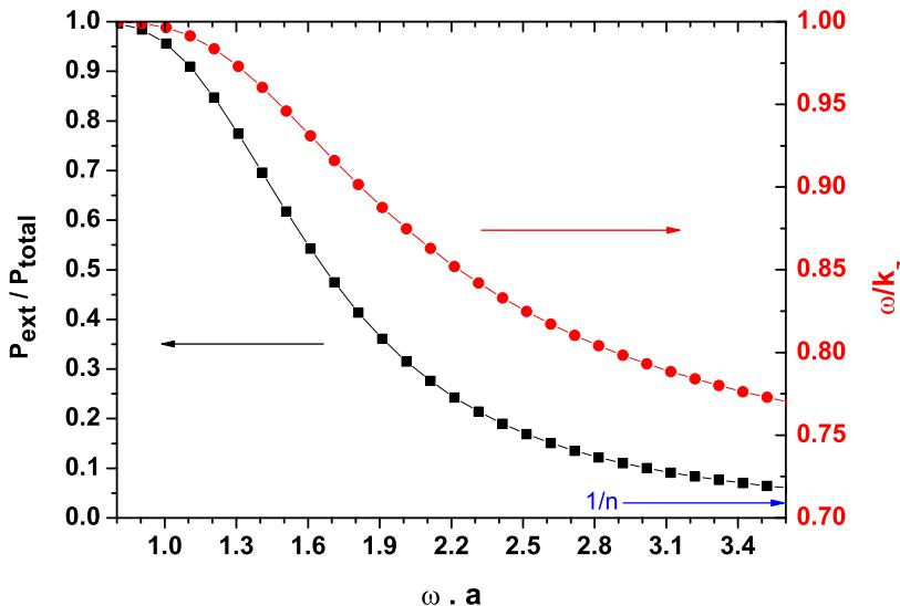
Fig. 2. Phase velocity  $v_{\text{ph}} = \omega / p$  (balls, right scale) and external fraction of the power (squares, left scale) for the  $HE_{11}$  mode.
