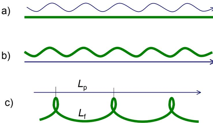
Fig. 6. Periodically bent particle trajectory (a), planar bent fiber (b) and helical bent fiber (c).  $L_p$  and  $L_f$  are the lengths of the curved or straight periods, for the particle and the fiber respectively.
