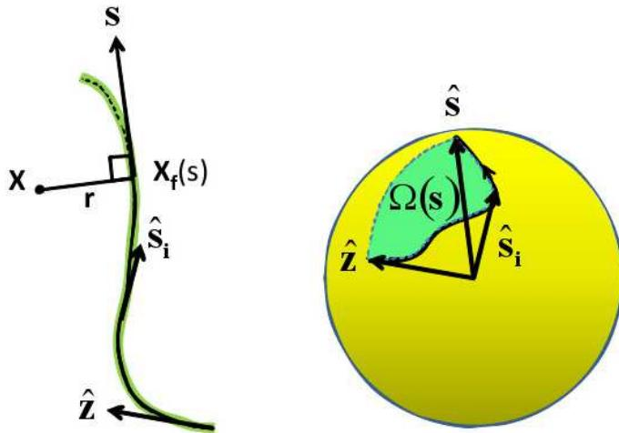
Fig. 3. Left: bent fiber and definition of  $X_f(s)$  and  $\mathbf{r}$ . Right: curve drawn by the extremities of successive tangent vectors ( $\hat{\mathbf{z}}, \hat{\mathbf{s}}_i, \hat{\mathbf{s}}, \dots$ ) on the unit sphere and definition of the solid angle  $\Omega(s)$ . The dotted arc of circle represents the “most direct” rotation,  $\mathcal{R}(\hat{\mathbf{z}} \rightarrow \hat{\mathbf{s}})$ , transforming  $\hat{\mathbf{z}}$  into  $\hat{\mathbf{s}}$ .
