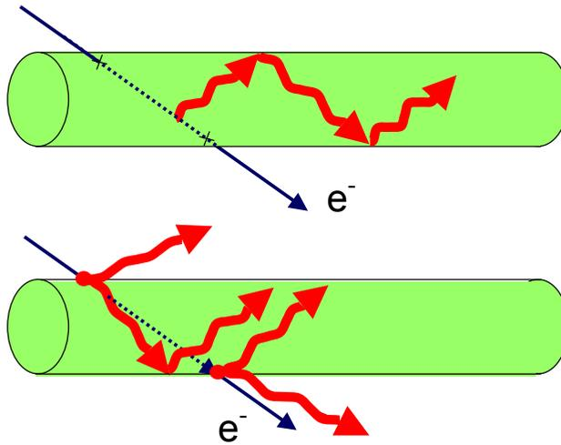
Fig. 1. Standard mechanisms of production of light inside a fiber, by an electron passing through. Top: Cherenkov radiation. Bottom: Transition radiation.
