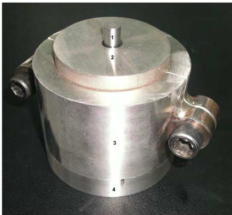
Fig. 2. The four-part dismantlable mold is shown in this picture: 1-punch, 2-four-section dismantlable block cylinder from high strength tempered steel, 3 - constricting clamp with twotightening bolts, 4 - support with groove for tungsten wire.
