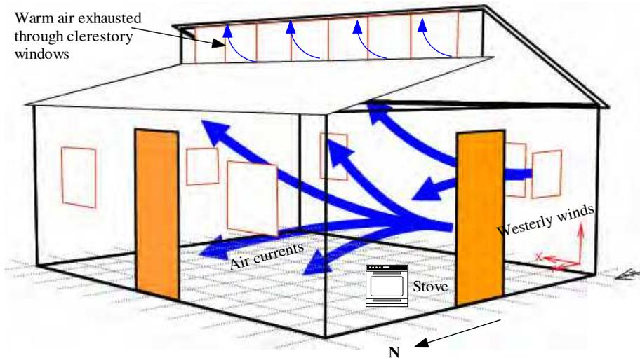
Fig. 6. Air current movements.
