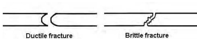
Fig. 7. Typical fractures of a ductile material and a brittle material.
