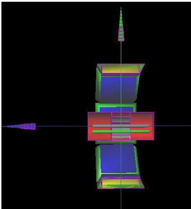
Fig. 2. Simulated 1-ring Albira scanner at a cross section at  $x=0$  plane. XYZ axes are coded as  $x$  in red (not seen in the image),  $y$  in green and  $z$  in blue. The green cylinder in the image represents the location of the tube with radioactive material. In the camera, green structures refer to the crystals.
