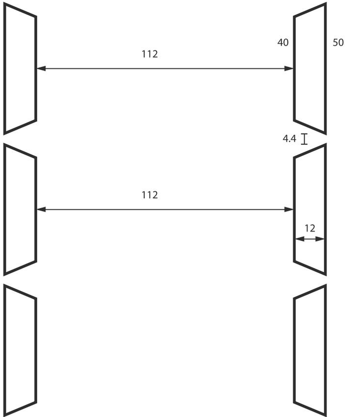
Fig. 1. Sketch of the dimensions of 2-rings camera in a horizontal plane. All dimensions are in mm. For 1-ring scanner the main difference is that the crystals are 9.8 mm thick, instead of 12 mm for 2- and 3-ring scanner. In simulations, 12 mm crystals were used, in actual production they are of 10 mm.
