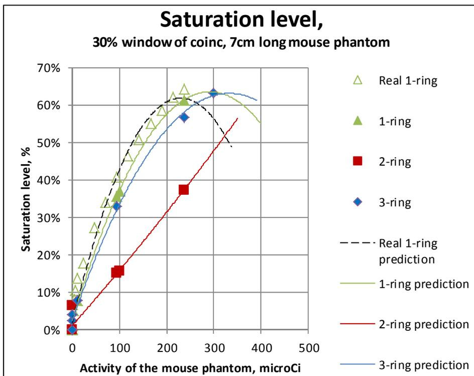
Fig. 9. Saturation levels for multiring scanners. For the 3-ring scanner with omitted 0<sup>th</sup> vs. 2<sup>nd</sup> ring coincidences, the saturation curve would be the same as for 3-ring geometry, as the efficiency is calculated as a fraction of valid coincidences for all activities. As the number of points for simulation is limited, we added the trend lines (2<sup>nd</sup> order polynomials) to look for expected evolution at higher activities.
