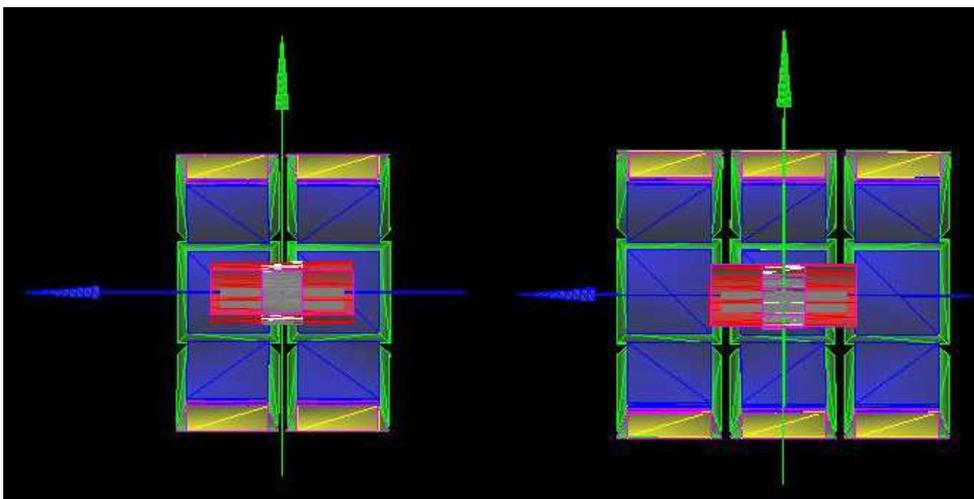
Fig. 7. The cross section view at around  $x=0$  of the simulated 2- and 3-ring scanner with the mouse phantom inside. The coding of the colors is the same as in Fig.2, disregard extra shapes inside the red mouse phantom.
