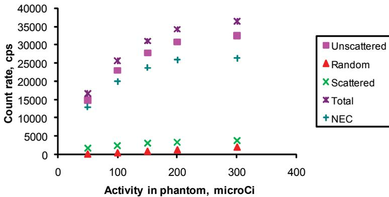
Fig. 6. Simulated NEMA mouse phantom rates for true unscattered, true scattered, random and total coincidences and noise equivalent counts (NEC) for 1 ring Albira scanner. Scatter fraction is constant and about 9% for the whole activity range. NEC has its maximum at 8.8 MBq of the described mouse phantom.
